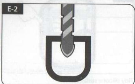
Drill a 25mm hole in the center of the tape marking
