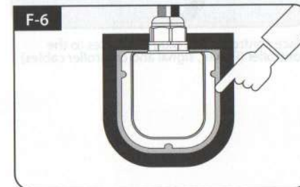
Connect cables to the ports of the antenna, remove masking tape and tidy silicone before dry
